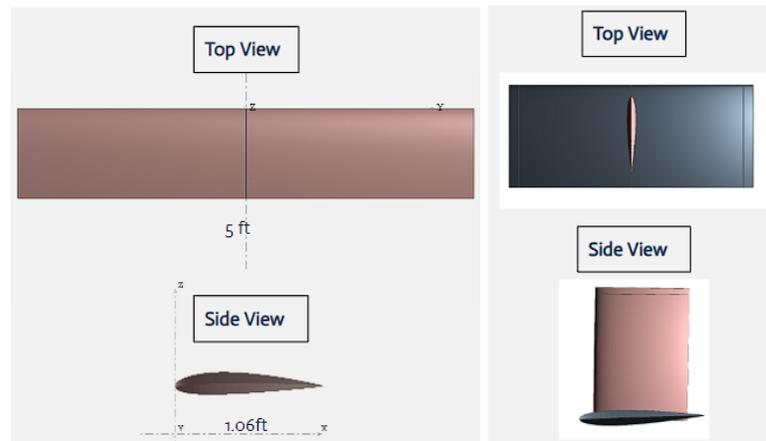
**Figure 16:** Modified XFLR5 views of Wing (Left) and Tail (right).
