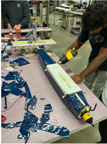
**Figure 34:** Monocoat application on fuselage.
