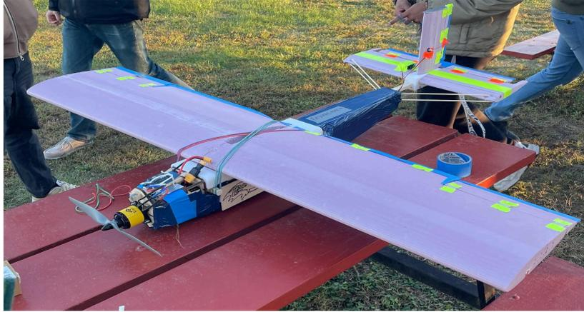
**Figure 27: Fully Assembled Plane Flight Ready**
